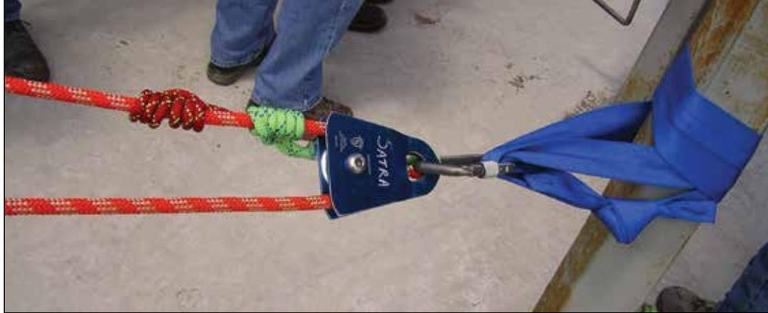
Setup for a horizontal lifeline and anchor point appropriate for side access into a grain bin. Photos courtesy of the Grain Entrapment Prevention Initiative.
