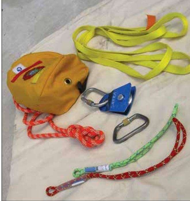
*Grain handlers need to provide employees with kits that include harnesses, lifelines, connectors, and belay systems that can be used to rescue persons entrapped in a grain bin. Photos courtesy of Wayne Bauer.*
