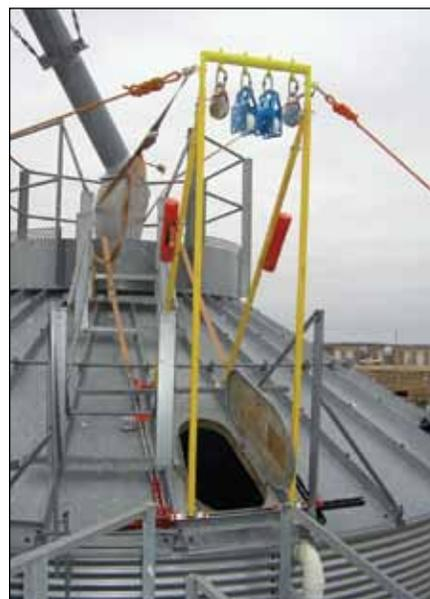
So-called "Aspen Lift" unit under development on the Oklahoma State University campus is designed to fit on steel tank roofs with slopes up to 45 degrees for extracting entrapment victims and rescuers. After testing is completed, plans are to make the lift available to the grain industry. Photos courtesy of Triangle Insurance Co.
