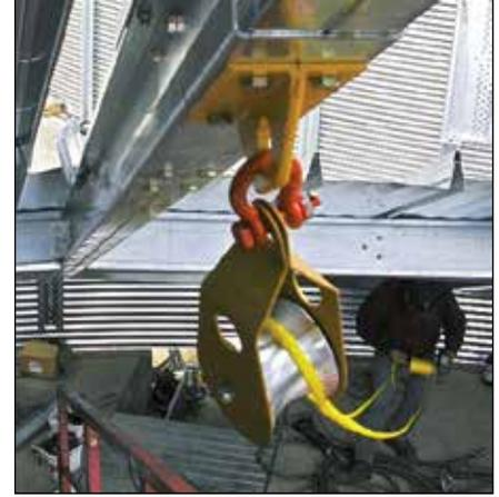
*Knot passing pulley developed as an anchorage at Star of the West Milling Co. This version is designed for 72-foot-diameter bins.*
